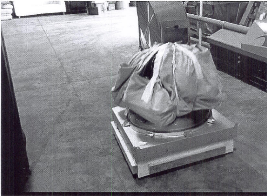
Photo No. 3: After impact of the 700 lbf static load from 2 foot drop height
