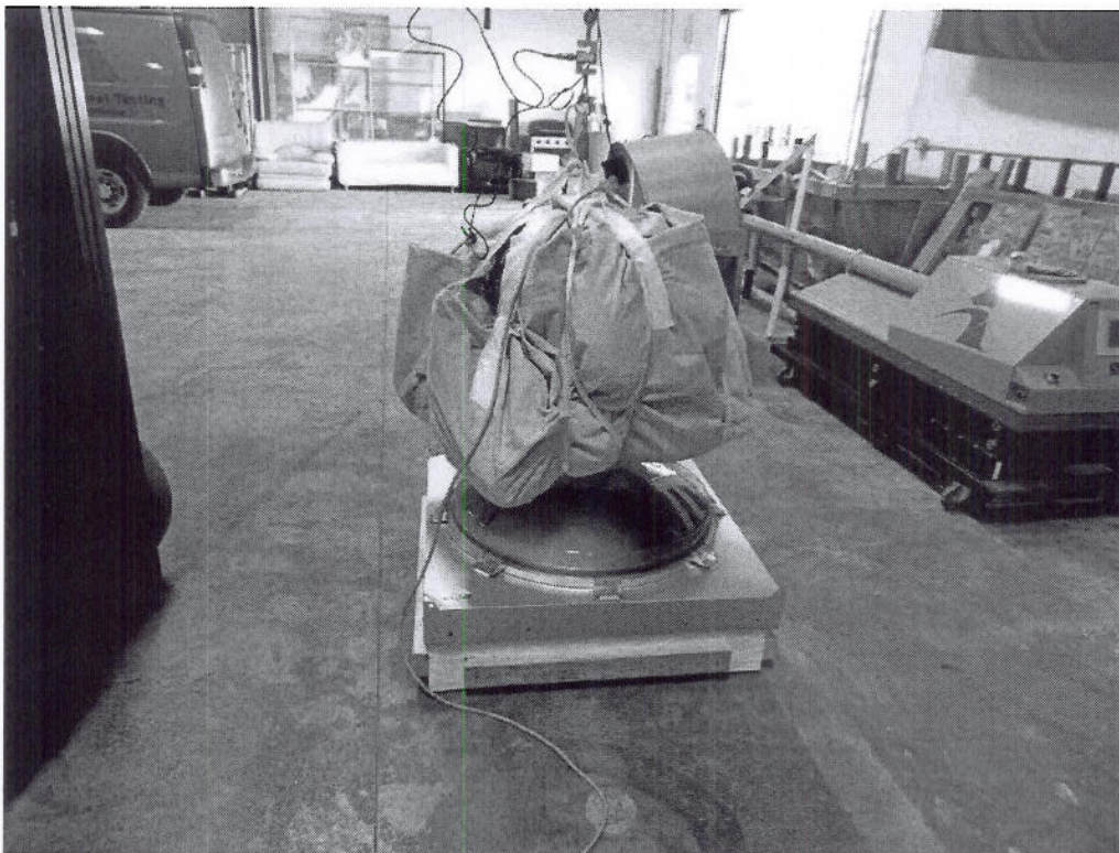
Photo No. 2: Test Specimen prior to application of the 700 lbf static load
