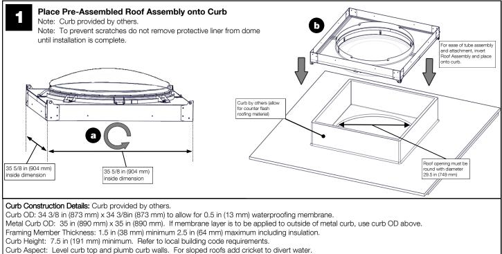
Curb Aspect: Level curb top and plumb curb walls. For sloped roots add chcket to divert water.
